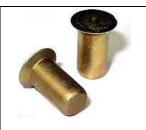
These NAS1097 rivets features for example a 1/8" diameter shank with a head size that of a 3/32" rivet. Perfect when rivet hole becomes enlarged requiring the next diameter up with the same head size as the original rivet.
